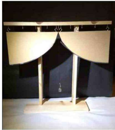
Figure 4: Photograph of Main Apparatus (Tautochrone)
